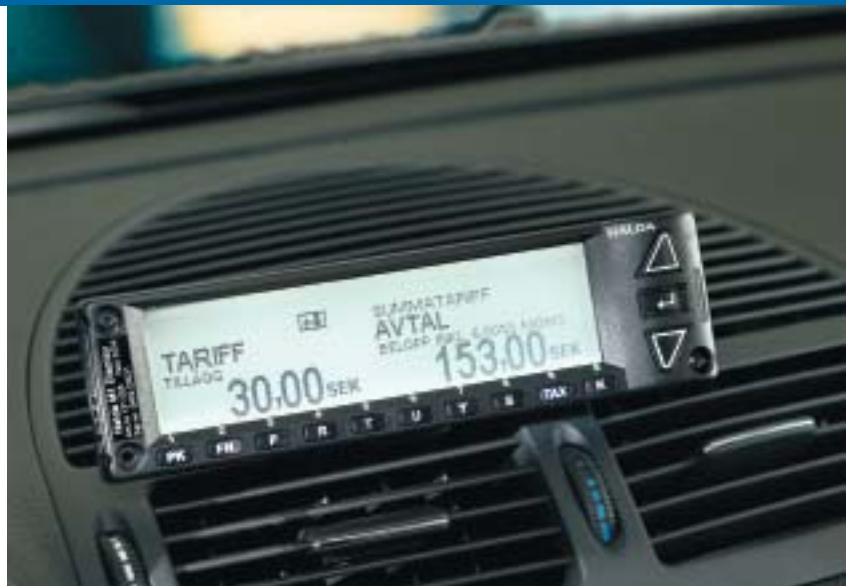
The taximeter is small and slim (176 x 23 x 50 mm) and weighs 200g.
