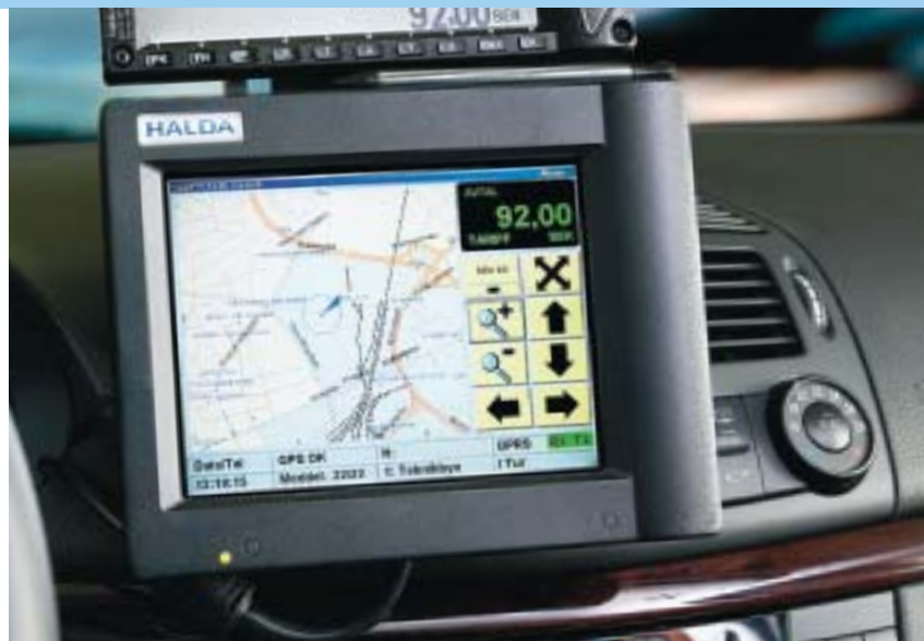
The computer screen (185 x 145 x 32 mm) weighs 725 g.
